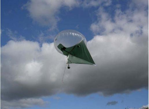
Launched within 20 minutes, a 14ft long, 11 cubic metre (385cu feet), Skyhook Helikite carrying gyro-stabilised pan/tilt/zoom video camera can provide continuous, long-term aerial surveillance over many miles. Manpower needed is just one. Running costs are minimal.
